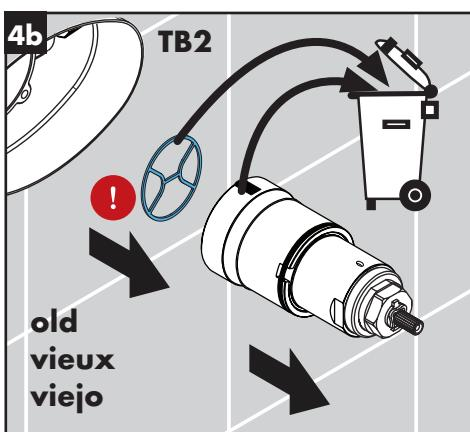
! The blue sealing gasket from the old cartridge MUST be removed from the rough valve. If it is not removed, damage to the new cartridge will result.
