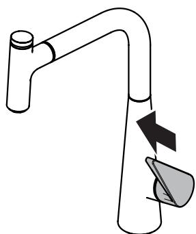
Use the lever to open and close the faucet and to set the desired temperature.
