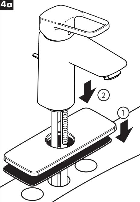
**Note:** The base plate is intended for use on a sink that is drilled for a 4" (100 mm) centerset faucet. Installation of the base plate on a sink drilled for a single-hole faucet is optional.
