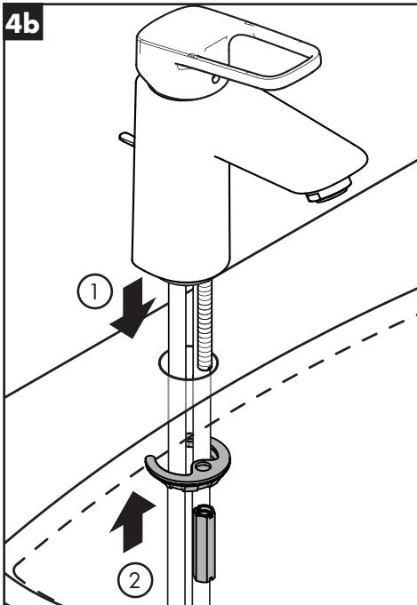
Install the washer and the mounting collar.
