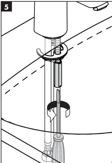
Tighten the collar using a flat head screwdriver.
