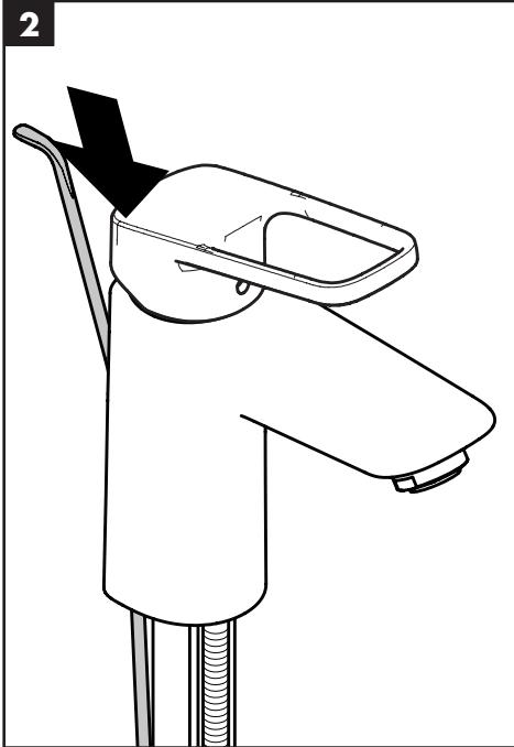
Install the drain pull rod.
