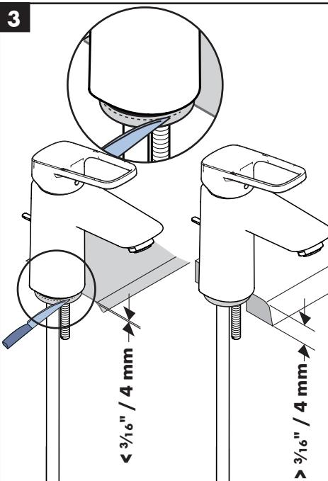
If the mounting surface is less than  $\frac{3}{16}$ " (4 mm) thick, trim the centering ring.
