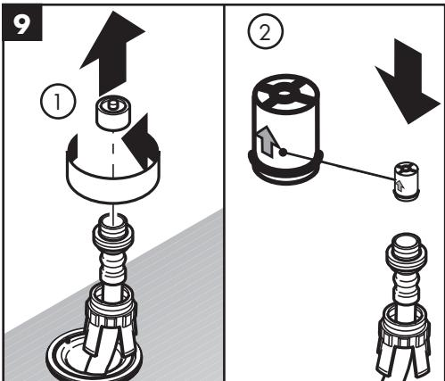
(1) Remove the brass plug and nut from the high pressure hose.
