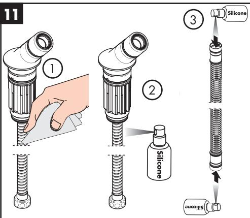
Lubricate the handshower hose using silicone spray.
