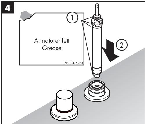
Lightly lubricate the o-rings on the diverter using white plumbers grease.
