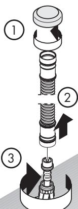
(1) Remove the plaster shield from the Secuflex hose.
