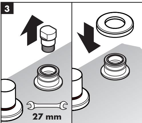
Remove the plug from the diverter housing.
